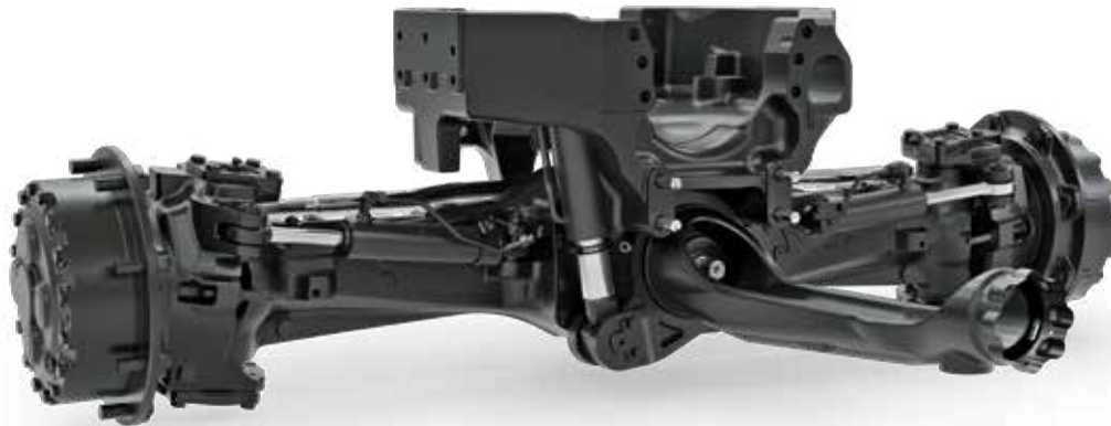
Front axle suspension works in both directions: more comfort, better traction and safety.
