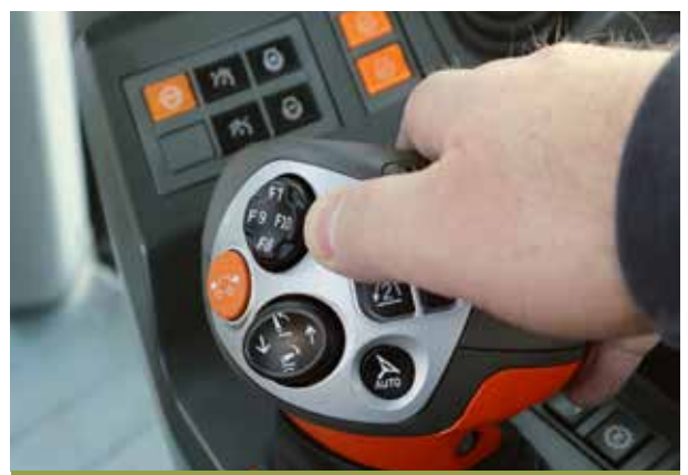
When the functions are programmed in the tractor's Isobus terminal, start / stop and quantity control +/- can be operated via the joystick.
