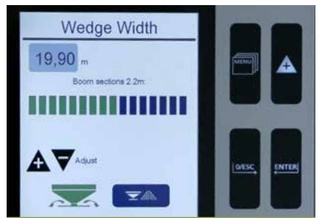
On remaining areas with asymmetrical tramline distances, an increased precision is obtained, as the section width is reduced.
