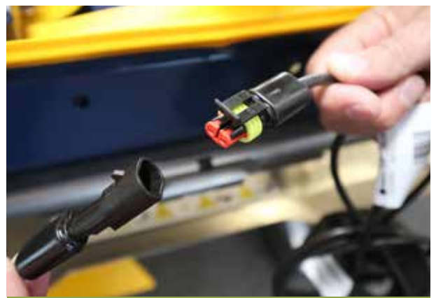
Well protected. The wiring loom is fitted with "Super Seal" plug connections that have IP67 rating.
